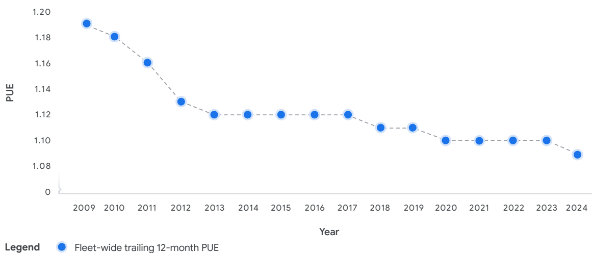
Figure 4. Energy efficiency (PUE) across Google data centers
